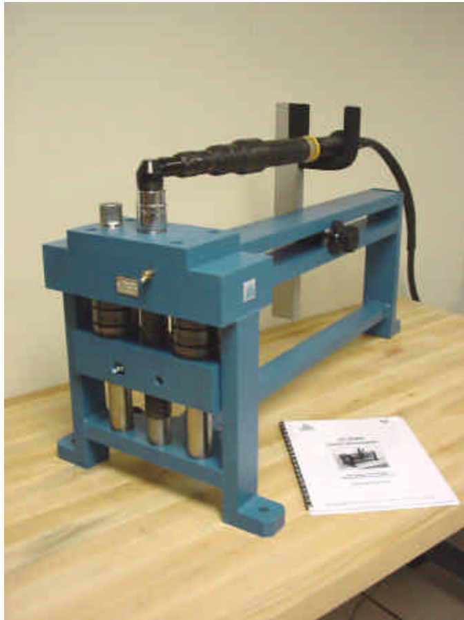
450 Nm Capacity Power Tool Testing Joint Simulator by RS Technologies
