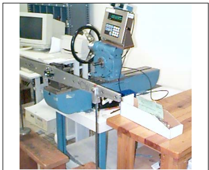
200 lb-ft Torque Calibration Stand
